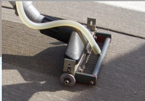
Suction port with pre-wetting nozzles
