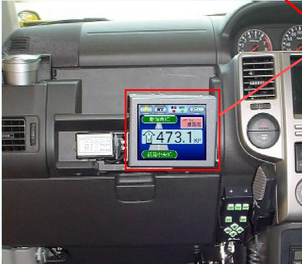
The new snow vehicle position monitoring system
