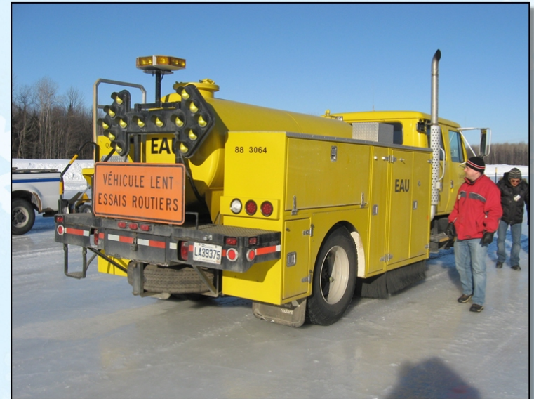
« Sideway-force Coefficient Routine Investigation Machine » (SCRIM)
