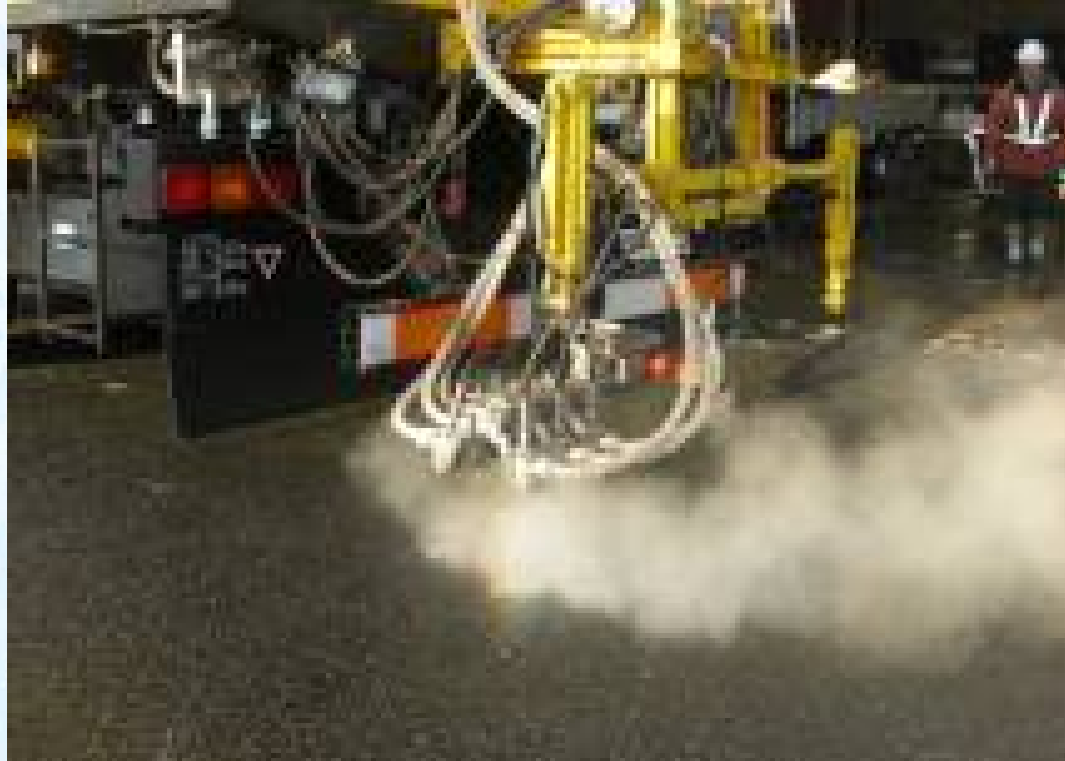
Fig.15-The cavitation jet being emitted from a swinging nozzle
