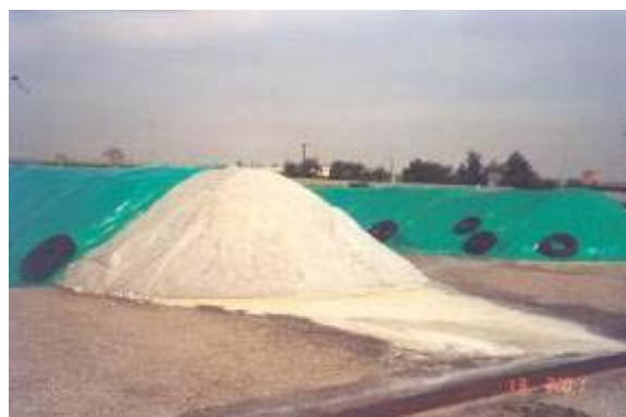
Figure 1-Salt in protected piles that has clearly been washed away
