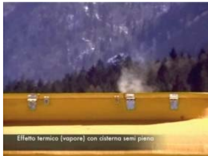
Figure 2 – Thermal effect (steam) with half-full tank after approx. 1 hour of work
