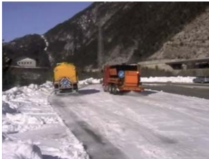
Figure 1 – Field comparison between tankers containing solutions of hot and cold \text{CaCl}_2 . The difference in the de-icing effect of the hot solution (at left) is significant.
