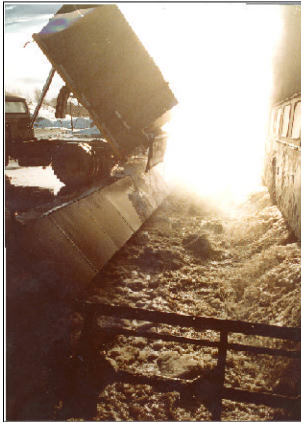
Figure 6 – A snow melter
