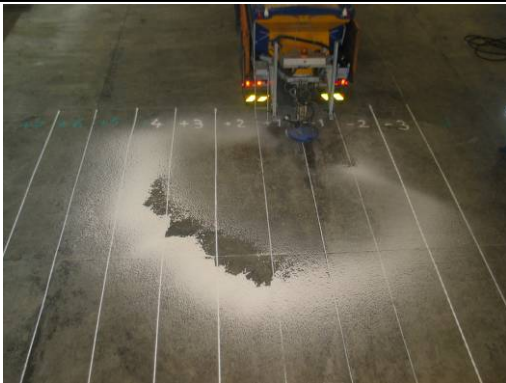
Figure 5: Distribution picture after stationary test
