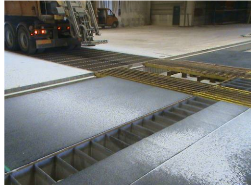
Figure 8: Measurement area with plates in the front and back of the measurement field
