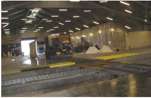
Figure 3 – Salt spreader runs over the measuring fieldweight cell
