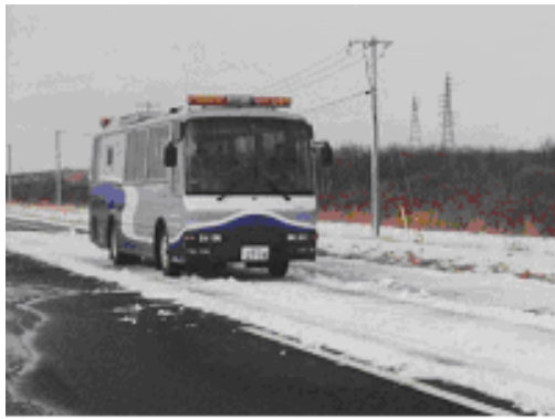
Photo 2 – Skid-resistance test vehicle
