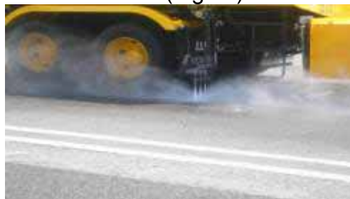
Fig.13-Lane marking cleaner attachment in operation
