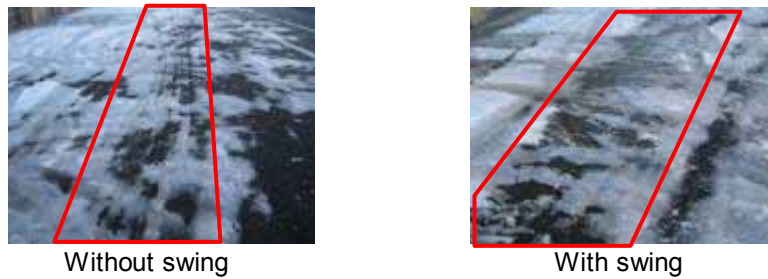
Fig.22-Break-up of snow and ice frozen hard onto the road surface
