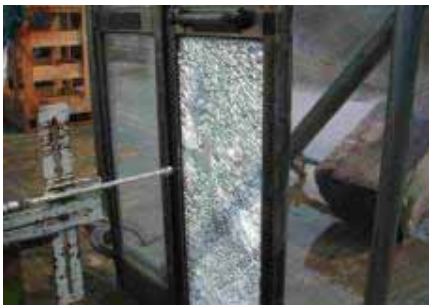
Fig.7-Failure test on tempered glass (8mm)
