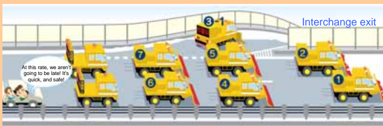
Fig.4-Diagrams outlining the old method of snow removal and multi-vehicle snow removal
