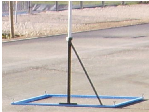
Photo 4 – The basis of support used to take pictures, measuring one square meter.
