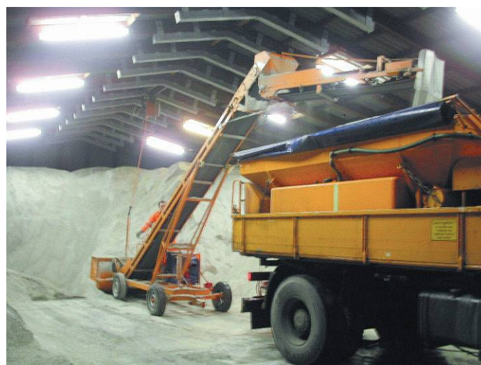
Figure 6 – Old loading technique per salt belt
