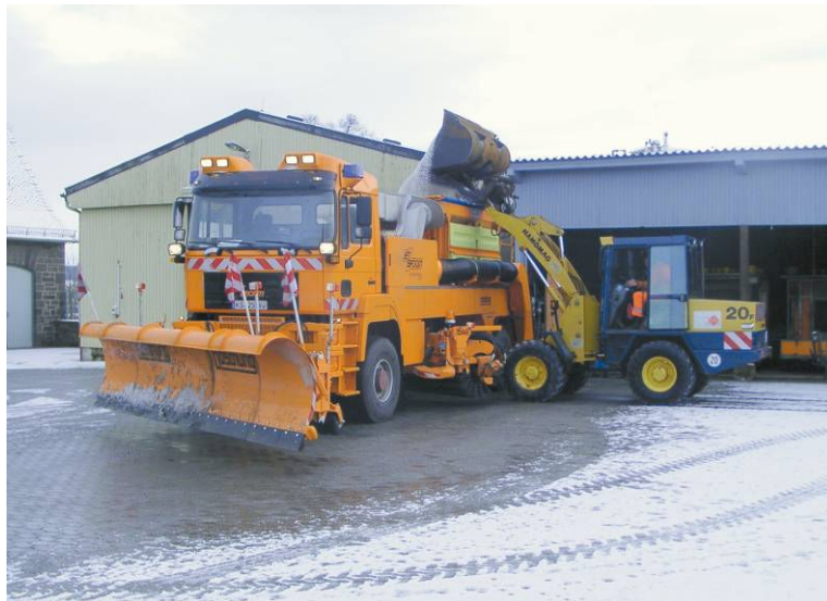
Figure 10 – loading from barn with wheel loader
