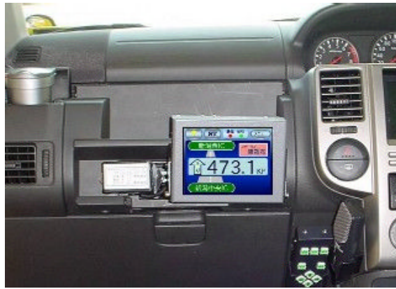
Fig.4 - The new snow vehicle position monitoring system
